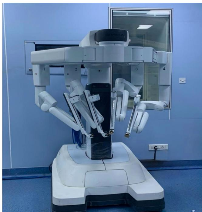
Figure 1. Robotic system da Vinci® Xi™
